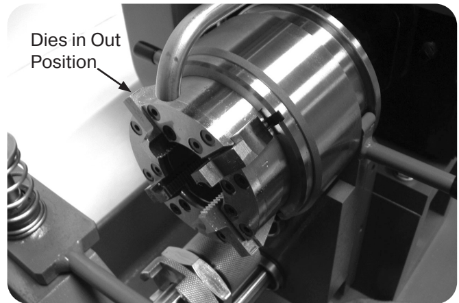
Figure 8 Moving die head to extreme position for chaser insertion by pressing head release lever
